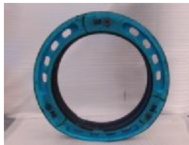
After 100 km load test with Ø 50 km/h
