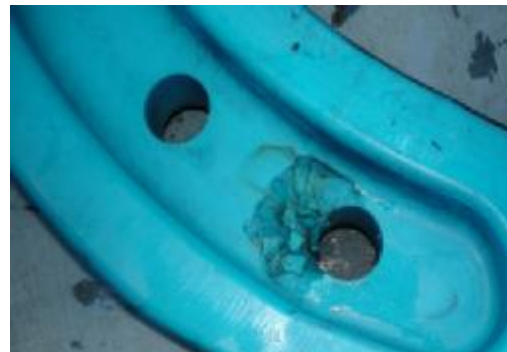
System after firing with NATO-Kaliber 7,6 bullets
